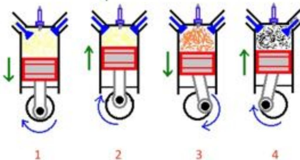
! Intake/Suck: a mixture air and gas is sucked into the cylinder (down)
